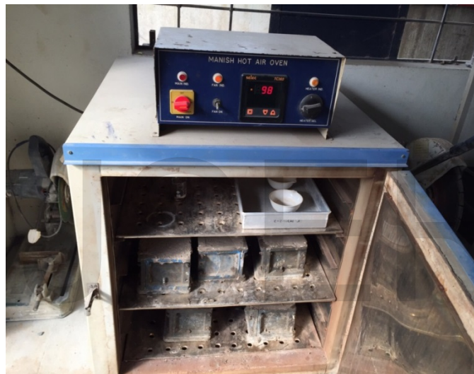
Fig- 2 :Specimens are placed in the oven for heat curing
