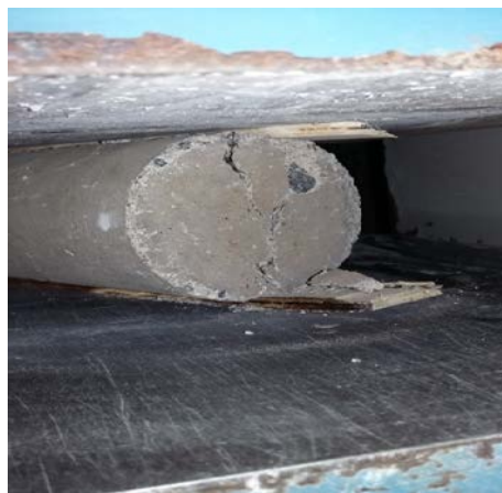
Fig-8 : Split tensile strength testing on cylinder.
