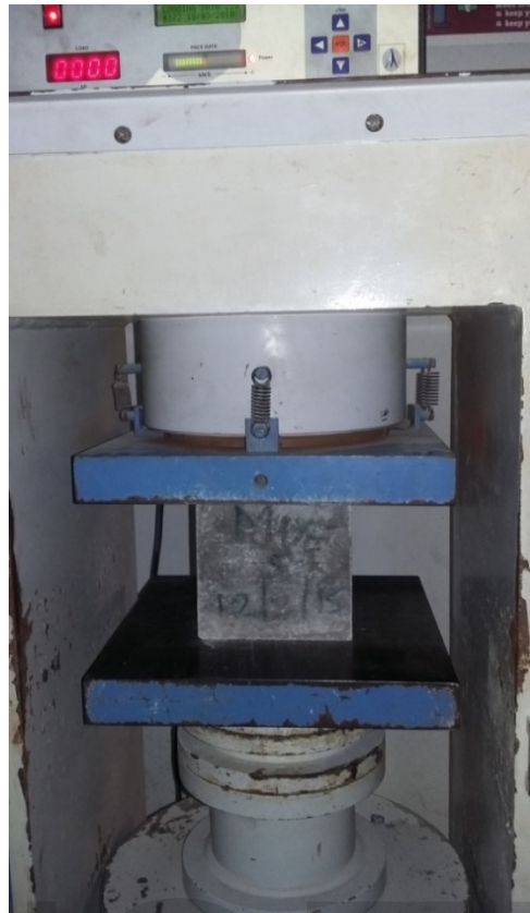
Fig -10: Compressive strength testing on Cubes of size 150mmx150mmx150mm
